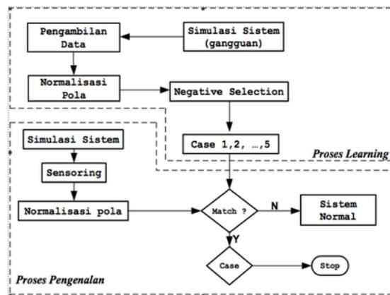
Fig. 1. Flowchart of a short circuit detection system on a distribution channel using AIS
