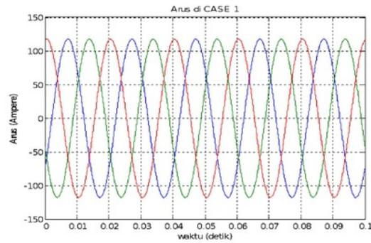
Fig. 2. Current signals in normal conditions
