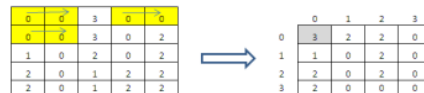
Fig. 7. (a) The image with 4 levels of grey, (b) GLCM at a distance of d = 1 , at 0^\circ
