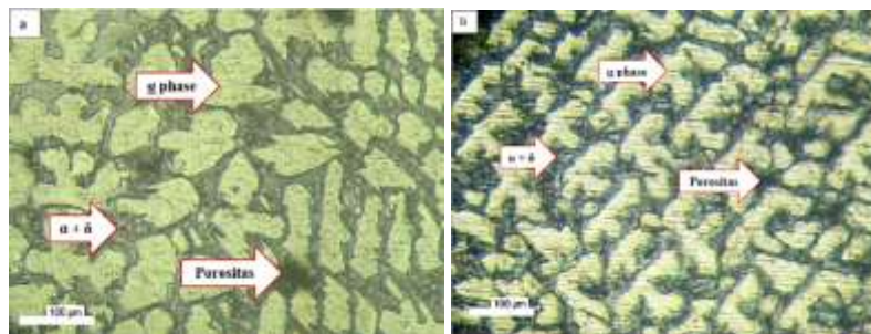
Gambar 19. Struktur mikro Cu25wt.%Sn (a) T_{s1} = 1000^{\circ}\text{C} (b) T_{s1} = 1100^{\circ}\text{C} sand casting .
