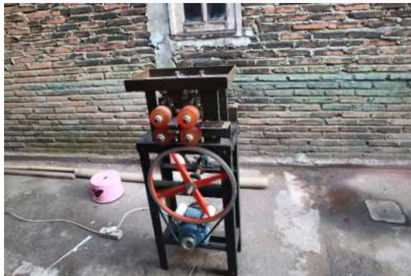
Figure 5. Shaved and Slitting Machine Resource: Researcher document
