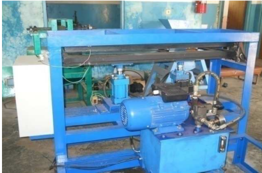
Figure 8: Automatic press machine with pneumatic system based PLC
