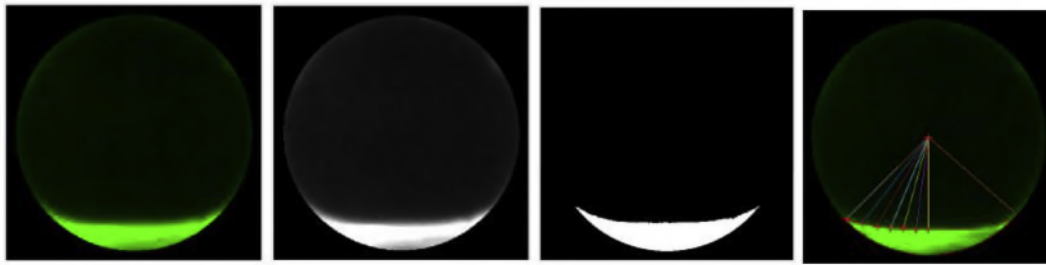
Fig. 6. The example of image processing steps: a. Cropping image, b. Grayscale image, c. BW image, d. Wetted wall angle dan perimeter plotted at the original image.
