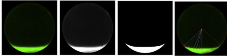
Fig. 6. The example of image processing steps: a. Cropping image, b. Grayscale image, c. BW image, d. Wetted wall angle dan perimeter plotted at the original image.
